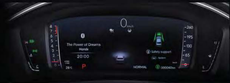
10.2" Interactive TFT Meter Cluster with Customized Display Setting
